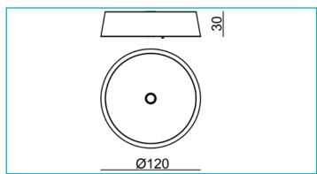
Housing Material Die-cast aluminium
