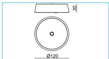
Housing Material Die-cast aluminium
